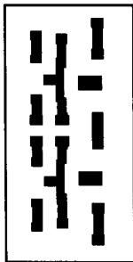
Fig. 3: Design and OPC corrected mask data for local interconnect pattern
